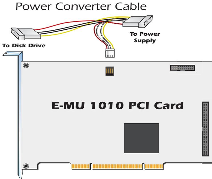
6. Plug the small connector into the E-MU 1010 PCI card as shown above. The connector is keyed and can only be inserted one way.
