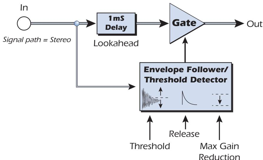
The Gate behaves exactly as a straight wire, except when activated by a signal level below the Threshold (with Lookahead Off).
