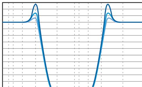
However, when the Highpass Freq parameter is lower than the Lowpass Freq parameter, the combined filter response is basically flat, since the passbands of each filter combine to admit the entire spectrum. An exception occurs when there is resonance added to the filters - you'll hear the resonant peaks as increased gain above the otherwise flat spectral response.
