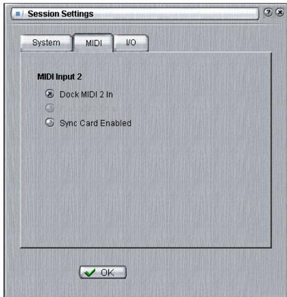
This option allows you to use either the MIDI In jack on the rear of the AudioDock or the Sync Card MIDI jack as a MTC Output. (The MTC Out only transmits MTC.)
