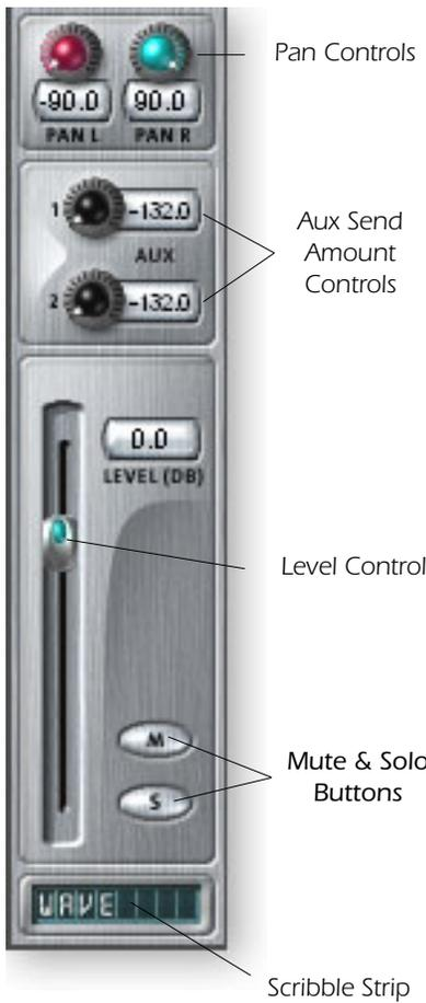
The **Pan** control comes before the Level Control and Aux Sends in the signal flow. On stereo strips we use an unconventional pan section with two pan pots – one for the left part of the signal and one for the right part of the signal. This feature allows you to independently position both sides of the stereo signal. A conventional stereo balance control only allows you to turn down one side or the other.
