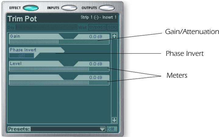
You might use a trim pot to boost or attenuate a send or return from an external effect, or to drive an effect device. Certain effects such as the Compressor, Distortion, and Auto-Wah are very level dependent and like to see a good, strong input signal. If you are working with a weak signal, you can improve the performance of these effects inserting a trim pot and boosting the gain.
