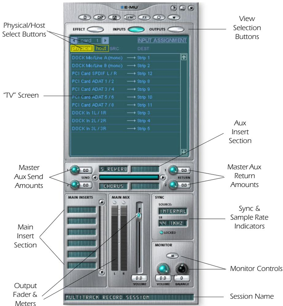
The main section contains all controls for controlling the main mix elements as well as a “TV screen” for viewing the parameters of the current selected insert.
