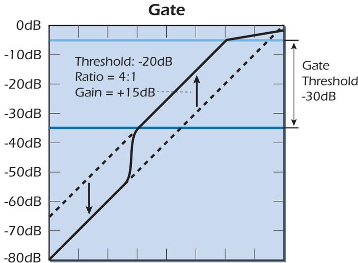
In this example, the Gain has been boosted by +15dB. The Gate cancels out the +15dB Gain boost below the Gate Threshold. Signal levels above the Gate Threshold will be boosted; signal levels below this point will not be boosted and will be 15dB lower in volume.
