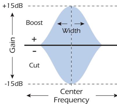
This single band parametric equalizer is useful when you just want to boost or cut a single range of frequencies. For example, if you just want to brighten up the lead vocal a bit, you might choose this EQ. This EQ offers up to  $\pm 15$ dB cut or boost.
