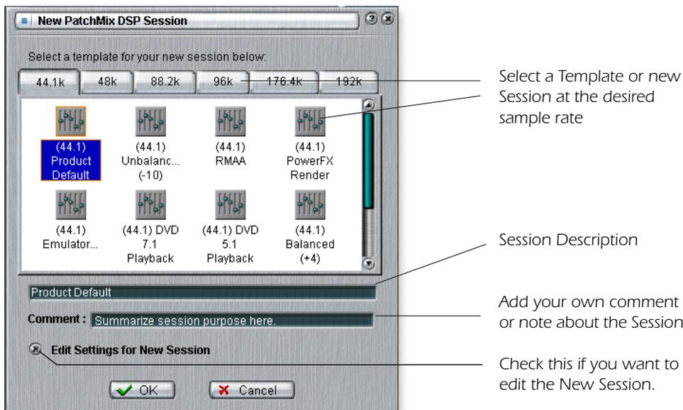
You can now select one of the factory template sessions. The factory templates are pre-programmed with specific setups such as audio recording or mixing. The selector tabs categorize Template Sessions into three groups based on sample rate, 44.1kHz/48kHz, 88.2kHz/96kHz, and 176.4kHz/192kHz.
