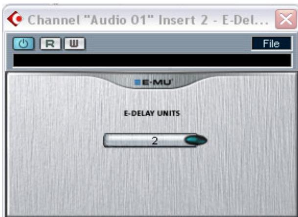
A host will support PowerFX and E-Wire's plug-in delay compensation if it supports the SetInitialDelay feature of the VST 2.0 specification.
