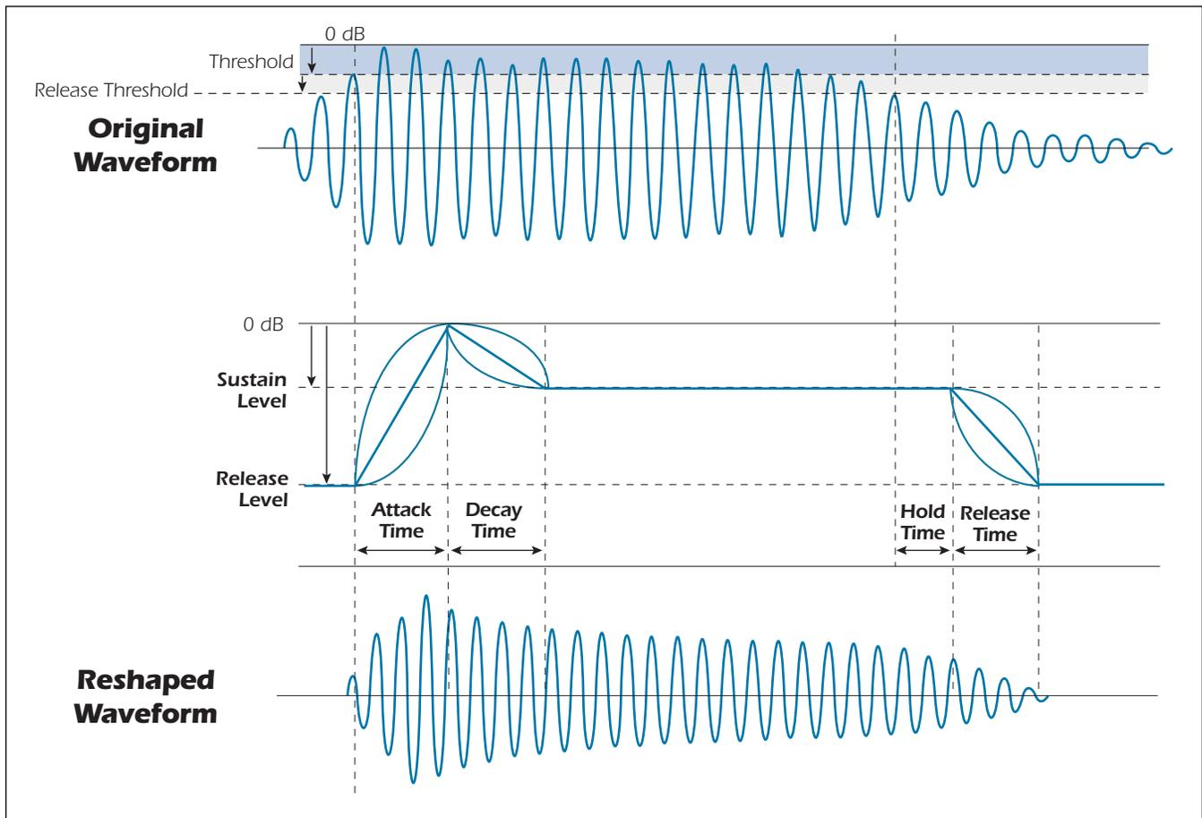
Attack, Decay and Release times are all adjustable, and the shape of each of these segments is selectable between exponential, linear, or logarithmic. An additional Hold Time can be used to extend the Sustain phase past the point where the signal has passed the Release Threshold.
