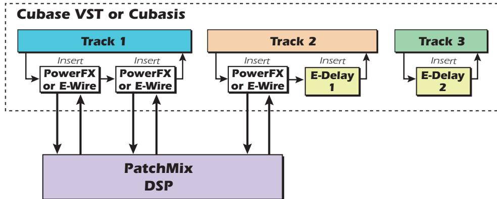
Since track 1 uses two PowerFX/E-Wire inserts, the delay of all the other tracks must equal two. Track 2 has one PowerFX/E-Wire insert and so adding one unit of E-Delay keeps it time aligned. Track 3 doesn't use a PowerFX/E-Wire insert and so it needs two E-Delay Units to remain in alignment.
