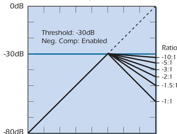
The diagram above shows the gain curves using a Threshold at -30dB and a range of negative compression ratios.
