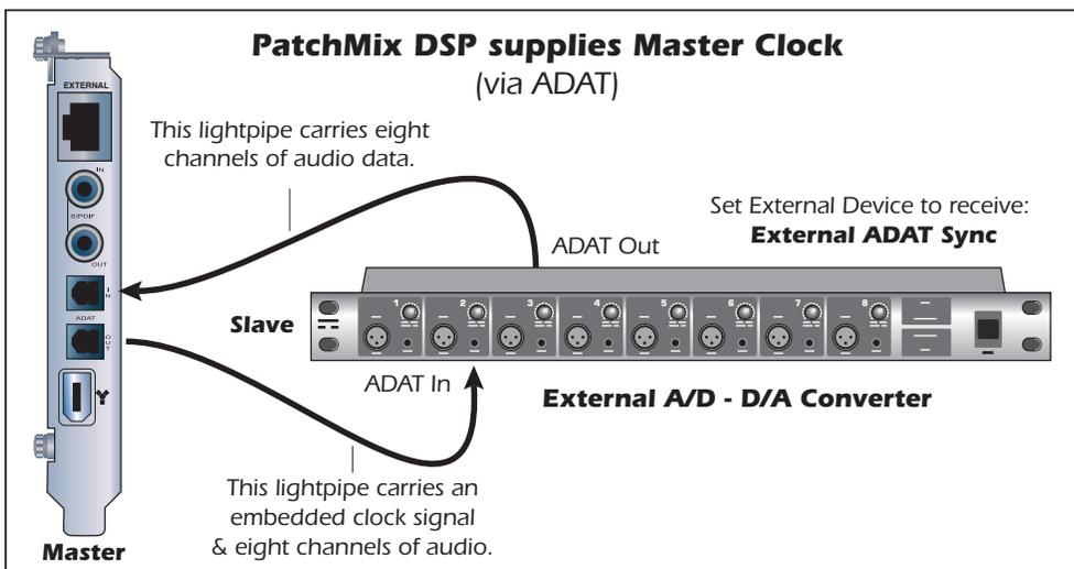
In the second example a second lightpipe is used to supply "embedded word clock", as well as eight channels of audio to the external A/D - D/A. The external device MUST be set to receive external clock via ADAT or the units will not be synchronized. The E-MU Digital Audio System is the Master and the external A/D - D/A is the Slave.
