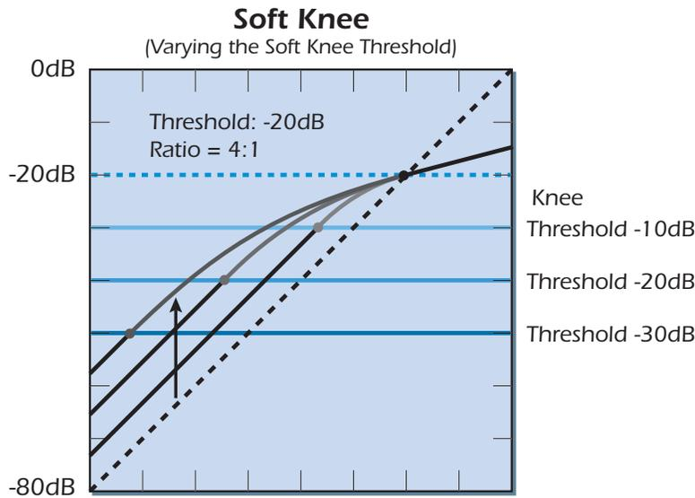
**This diagram shows the effect of varying the Soft Knee Threshold.** Compression is 1:1 (no compression) at the Knee Threshold and smoothly transforms into the selected compression ratio at the Compression Threshold. The upward arrow shows the additional gain added to signals below the Threshold.
