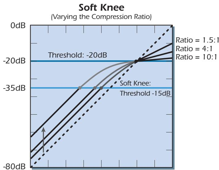
**This diagram shows the effect of varying the Compression Ratio** with a fixed Soft Knee Threshold. The knee transforms from a linear slope to the slope of the compression ratio over the Soft Knee Threshold area. The upward arrow shows the additional gain added to signals below the Threshold.
