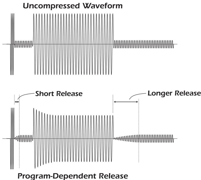
With Auto-release turned on, the release time becomes longer after an extended period of compression.
