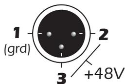
Balanced dynamic microphones are not affected by phantom power. An unbalanced dynamic microphone may not work properly, but will probably not be damaged if phantom power is left on.
