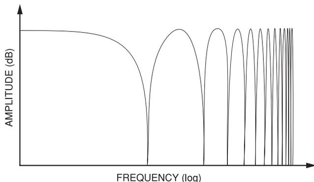
A low frequency oscillator is included to slowly change the delay time. This creates a rich, sweeping effect as the notches move up and down across the frequency range. The amount of feedback deepens the notches, intensifying the effect. You can invert the feedback signal by choosing a negative feedback value. Inverting the feedback signal creates peaks in the notch filter and deepens the effect.
