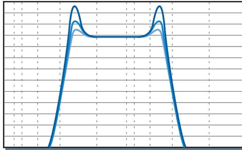
However, if the Highpass Freq parameter is greater than the Lowpass Frequency parameter, the passband effectively disappears, since the part of the spectrum which is above the highpass and below the lowpass is non-existent. As a result, you'll hear a rapidly attenuating bandpass response as the corner frequencies diverge.
