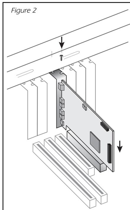
5. Align the E-MU 1010 PCI card with the slot and press gently but firmly down into the slot as shown in figure 2.
