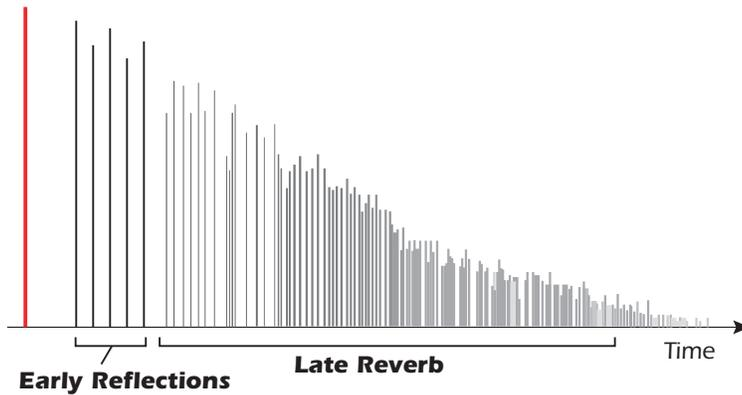
After a short pre-delay period, the echoes from the closest walls or ceiling are heard. These first echoes, or early reflections, vary greatly depending on the type of room. Some time after the early reflection cluster ends (late reverb delay), the late reverberation (a dense cloud of complex wall reflections) begins and decays according to the time set by the Decay Time parameter.
