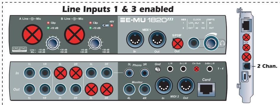
At the 176.4kHz or 192kHz sample rates, you sacrifice S/PDIF, line input 3, and line output 3. ADAT optical is reduced to two channels. You can choose one of the following options:
