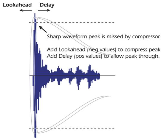
At positive values, the signal path delay is zero; instead, a delay of up to 50 milliseconds is inserted into the sidechain path containing the level detector. This delay can be used intentionally to cause the compressor to miss signal peaks, retaining the “punch” and
