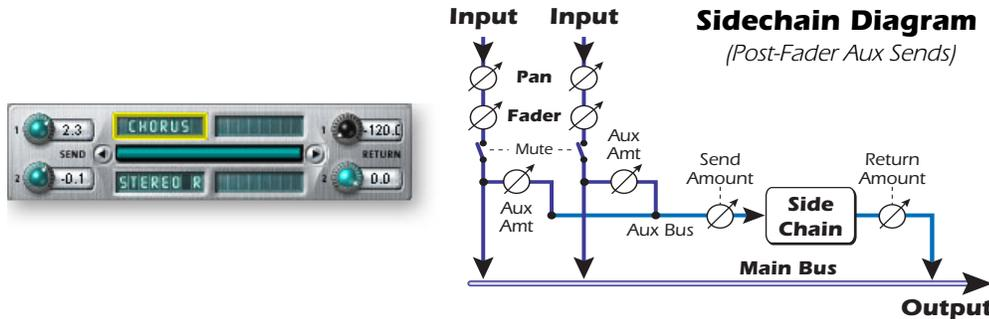
You can also use the Auxiliary Sends as two extra mix buses. By turning the Aux Return amount all the way down and dropping an Insert Send into the chain, you can send the Auxiliary bus to any output you wish. See [“Insert Section”](#) for more information.,
