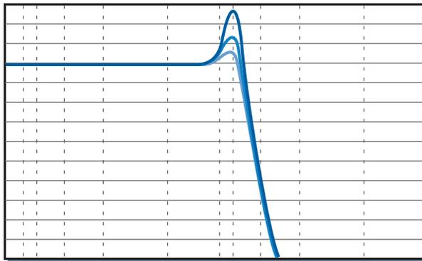
In this mode, the Lowpass filter can have up to a 48dB/octave rolloff slope. In this mode the Lowpass Rolloff, Lowpass Frequency and Lowpass Resonance parameters are available for editing the filter response.
