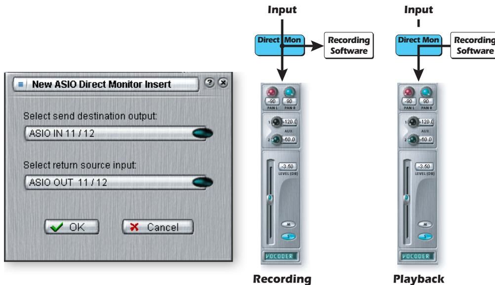
The Direct Monitor Send/Return also allows the recording application to control volume and pan. Normally when using direct monitor recording you'll want to control the volume and pan from the recording application. In this case, set the PatchMix DSP stereo pan controls hard left and right, mono pan controls to center, and the fader to 0dB.
