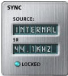
The Sync/Sample rate Indicators show the current session’s sample rate and whether it is internal or slaving to an external source. The LEDs indicate which sample rate is currently in effect. If an external source is being used, the Source display reads “EXTERNAL”.
