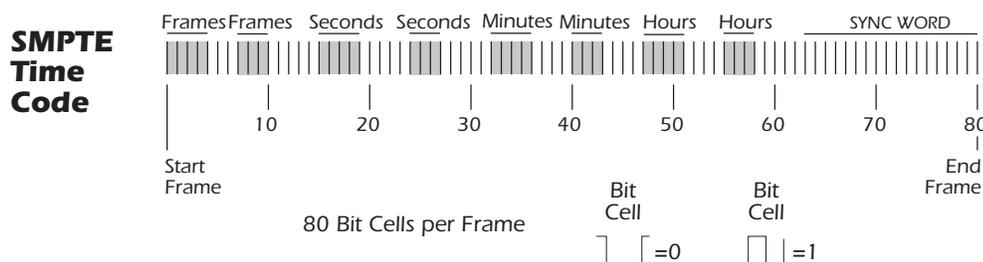
There are four types of SMPTE time code in general use: 24, 25, 30 frame-per-second and 30 drop-frame. In general, you should choose one rate (30 non-drop is common in audio) and stick with it for initial recording and later editing.
